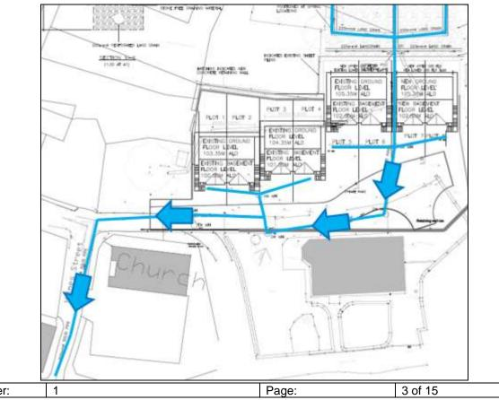
The development as amended would discharge surface water / land drainage into exactly the same culverted watercourse as approved under the original planning approval (ref: 2016/0630), albeit this time discharging into the watercourse approximately 45m further downstream to the west.
