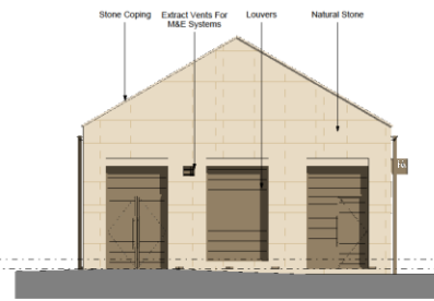
PROPOSED SOUTH ELEVATION Scale: 1:50
