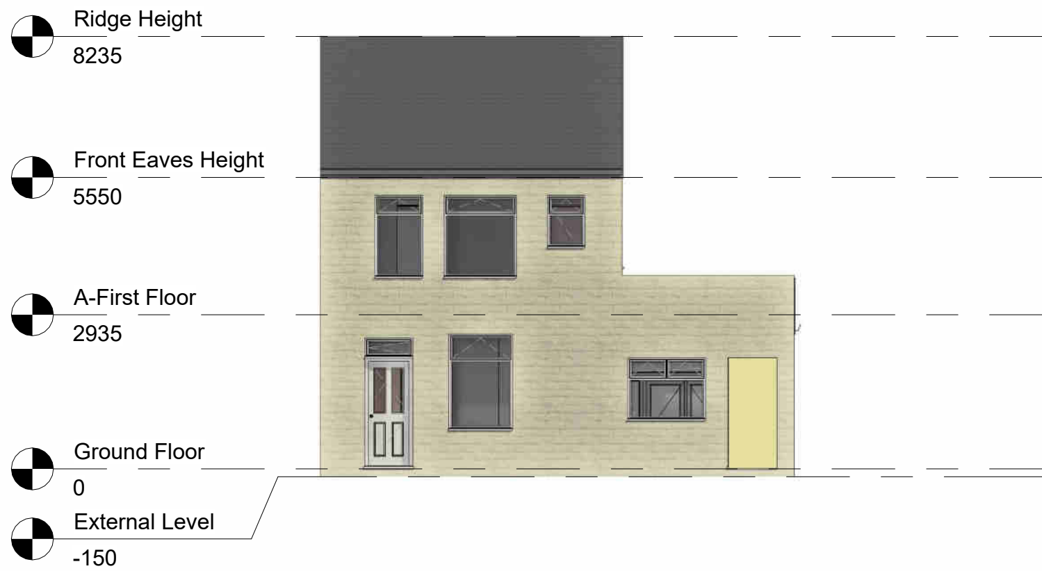
4 Existing Front Elevation 1 : 100
