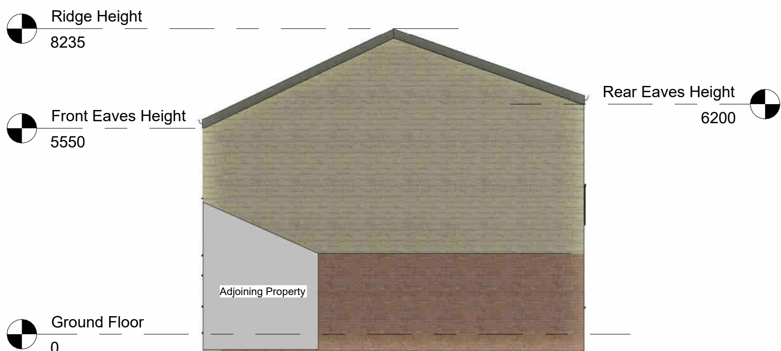
6 Proposed RHS Gable Elevation 1 : 100
