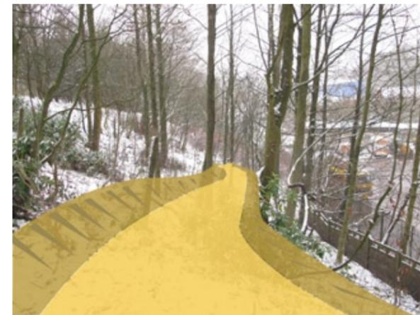
View showing path dropping away through the woods at a gradient of 1:20. If the soil is adequate the path can be cut through on a low bench
