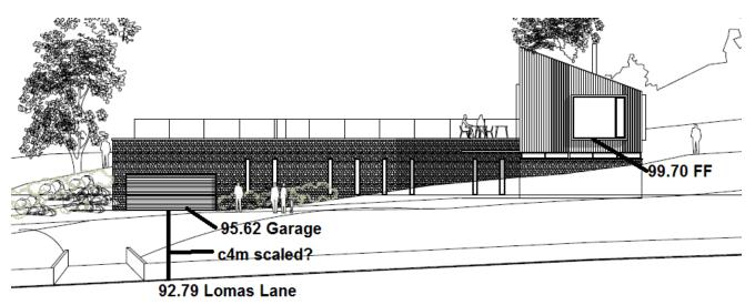
**5 Have levels changed?** 2005/0025 shows: Garage 95.62, Ground Floor 96.50, First Floor 99.70; but there are the same levels on the plans for 2013/0587. The applicant needs to clarify whether the proposed floor levels on 2013/0587 were, in relation to Lomas Lane, 1.2 metres higher.
