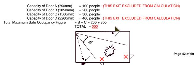
\* WELL SEPARATED: Fire exit separation is generally defined by the 45-degree rule. If from any point in a room, two exits cannot be included within a 45-degree angle, then they may be viewed as being well separated. The following diagram illustrates well-separated exits:
