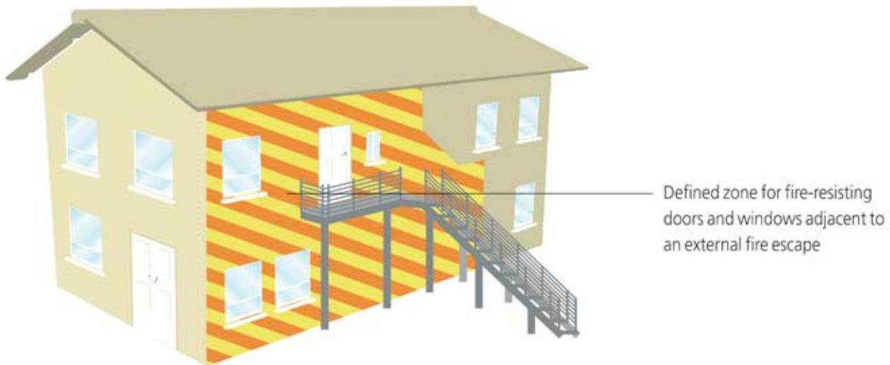
proprietary constructions and products are available which have been tested to these standards and have a valid test certificate demonstrating 30 or 60 minutes of fire resistance.
