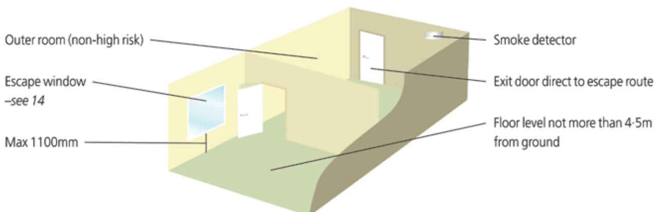
13.3 In all cases a suitable automatic fire detection and warning system should be in place (see paragraphs 22-25).
