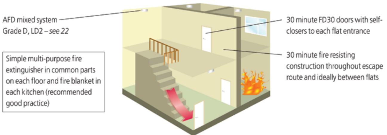
is the ideal, but on risk assessment there may be no requirement for additional fire-resisting separation between units providing walls and floors are of sound, traditional construction and additional compensatory detection is fitted.
