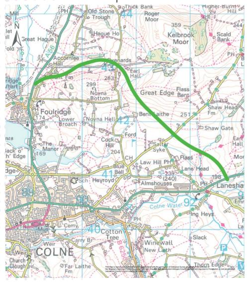
The Green Option would create an east - west bypass to the north of Colne and Foulridge if delivered in conjunction with a southern bypass option. The Green Option starts from a junction on the A56 to the north of Foulridge, which would link with a southern bypass option. It would finish at a new junction with the A6068 to the east of Laneshaw Bridge. The route is 4.6km long and has 6 structures and 3 intermediate junctions.
