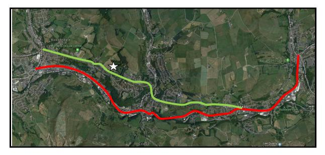
The site location highlight is along the Newchurch Road/Booth Road corridor and the flows are substantially lower than the A681 corridor, in effect the east west movements can take place with no interaction other than at the Toll Bar mini roundabout.
