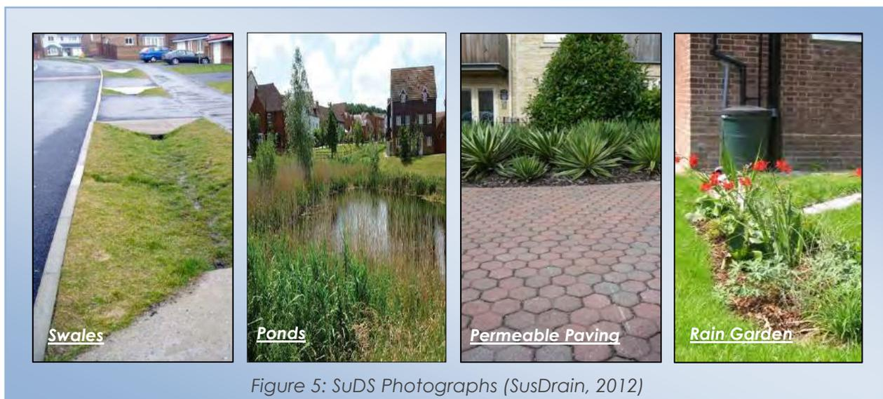
5.3.4 Promoting SuDS to deal with surface water at the source, will limit the required attenuation and in turn reduce the volume of surface water in the nearby watercourse and sewer infrastructure. There may be the potential to utilise SuDS features for conveyance/attenuation of surface water flows within the proposed drainage strategy, opposed to the traditional below ground storage methods. Detailed design
