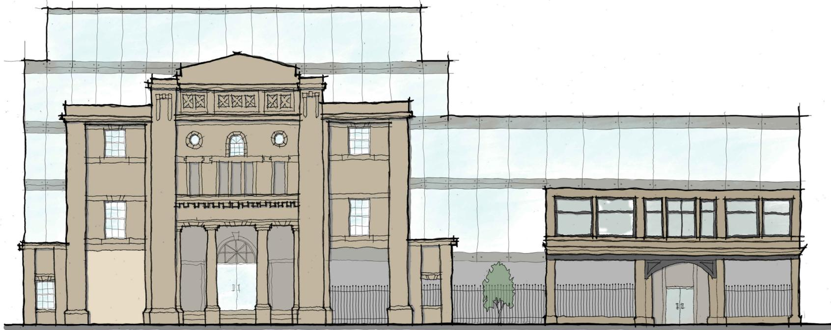
Proposed Northern Elevation - Retained Facades
