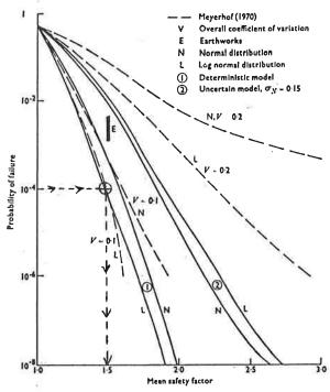
Fig. 16. Relationship between safety factor and probability of failure
